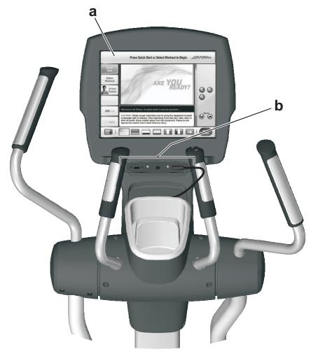
**a. Touchscreen Display:** The Touchscreen Display (the LCD screen) allows the user to choose, set up, and monitor a workout.
